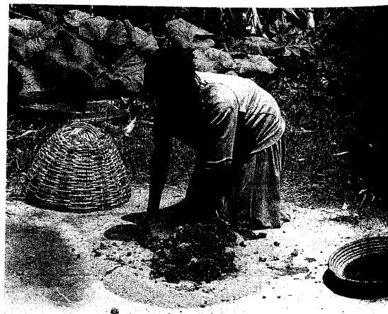
Fig. 11.7 Tabita mixing clay, grog, and water.
