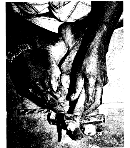
Fig. 9.9 Abib using the cow-horn die to shape silver beads.
